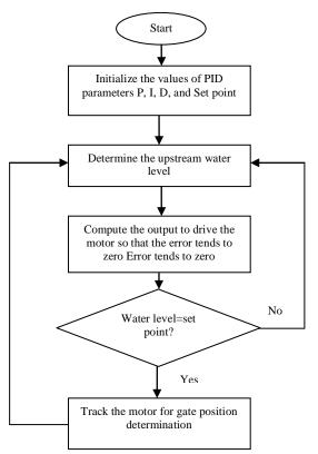
Fig 2: Flow chart of canal automation system
