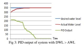
The figure 3 shows the PID output generated by first instantiation of PID algorithm when desired water level (DWL) is greater than actual water level (AWL). The above plot clearly shows that with the positive error the designed system achieves the zero steady state error within short time interval. The PID output is a function of the error generated between the two water levels.
