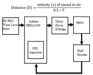
Fig 1: Block Diagram of canal gate automation system
